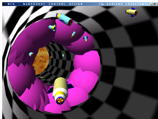
Figure 6: Vein inside view without the red blood cells. The target plaque is represented by the pink spheres surrounding the vessel wall. The nanorobots swim in a near-wall region searching for the atherosclerotic lesion.
