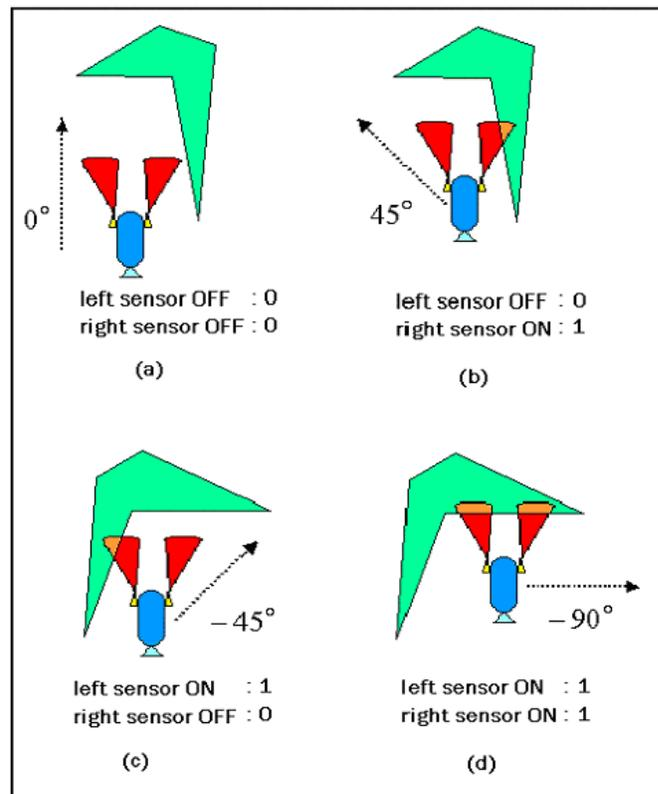
Fig. 4. Sensor-based navigational behavior.
