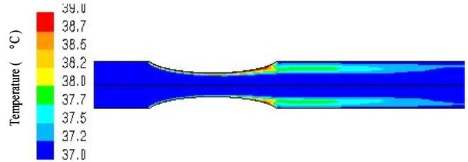
**Figure 4:** Blood temperature distribution in the systolic phase of a 50% diameter stenotic segment of the LAD coronary artery model (blood flows from left to right). Wall temperature at the stenosis region is set to 39°C.
